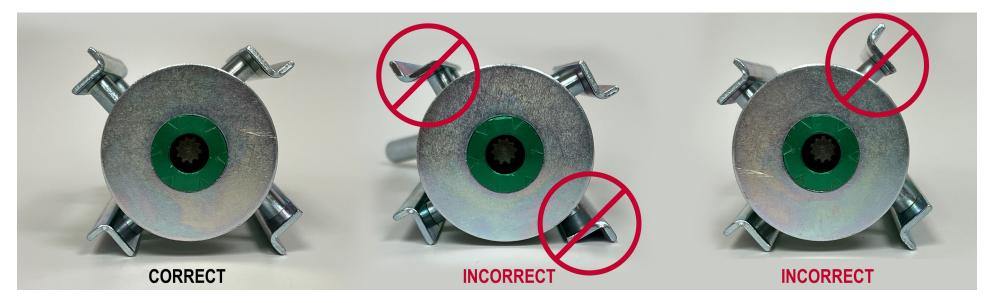
This image shows the correct and incorrect orientation of the racks from the bottom of the tool. If all of the racks are not facing the same direction you have a tool that was assembled incorrectly. **DO NOT USE THIS TOOL**. Contact us for a remedy. You may have a tool with 2 racks facing the wrong way or 1 rack facing the wrong way. Incorrect Rack Assemblies are circled. Typically the incorrect rack is holding a stone.
