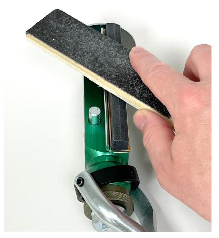
Correct any taper in stones by dressing with the abrasive paddle supplied.
