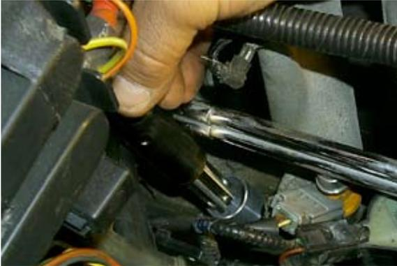
4. Insert tap assembly into stop tube and turn with 1/2" ratchet & extension until it bottoms out against the top of the stop tube. Then remove.
