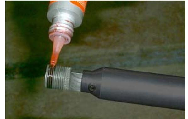
9. Apply a bead of thread sealant toward the bottom of the insert.
