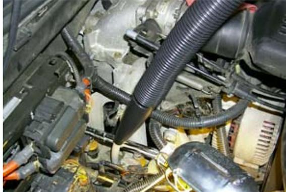
5. Use vacuum extension with a vacuum to remove aluminum shavings that have dropped into cylinder. Be sure to remove all shavings.
