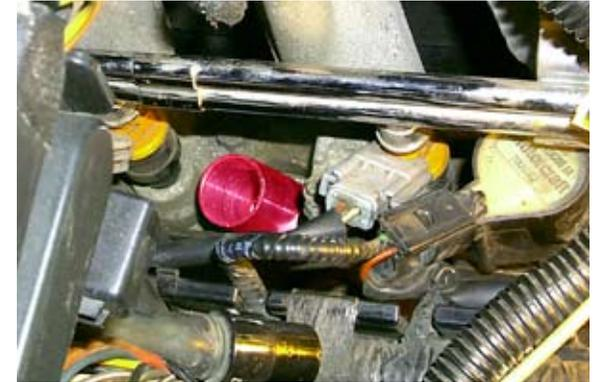
3. Place stop tube against the wall of the head so it lines up with the plug hole.
