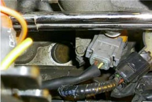
1. To begin, remove any obstructions. Turn crank so piston below damaged spark plug hole is down on the power stroke.
