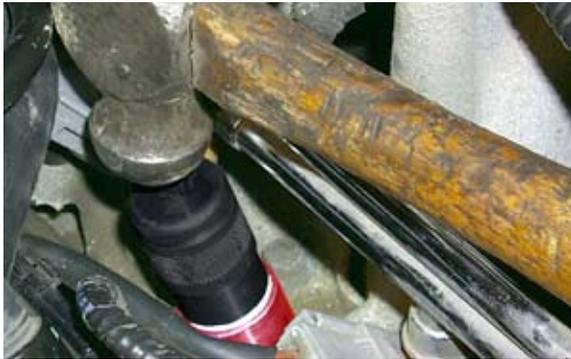
13. Place swedger in hole and strike with hammer until the white line meets the top of the stop tube. Do not over swedge.
