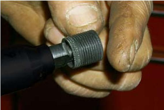
7. Thread the sleeve onto the inserting assembly. Serrations go on first and will hold the sleeve in place at the top of the tapped plug hole.
