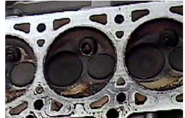
15. Now the plug can be inserted. It will line up exactly with the other plugs. In this photo the middle plug has been fixed with a sleeve.
