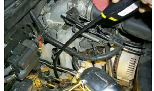
6. Use an inspection scope to make sure all shavings are removed from cylinder. Vacuum again if necessary. Start motor to blow out what you don't suck out.
