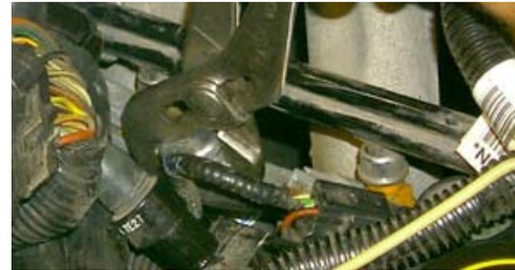
14. To remove swedger tap gently on the side of the swedger or use a flat blade screwdriver in top groove to pry the swedger from hole. You may also use pliers to twist the swedger out in hard-to-reach areas. Remove stop tube.
