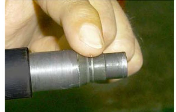
12. Apply grease or oil to the angle on the swedger assembly.
