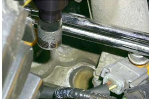
11. Screw the insert into hole by hand until head comes to within .060" of top of stop or until against stop.
