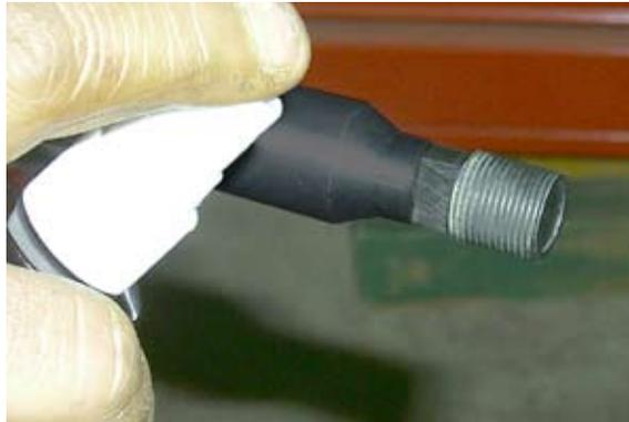
8. Spray the insert with the thread sealant primer.
