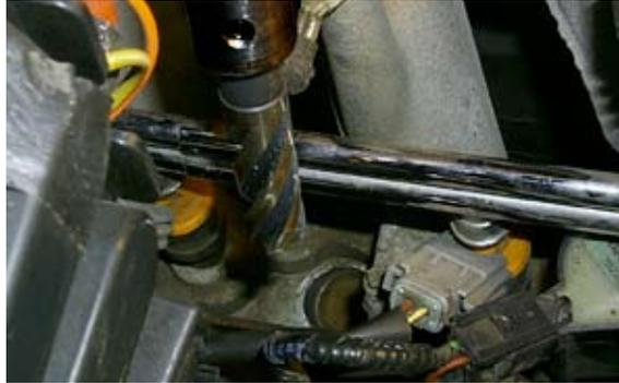
2. Use the drill assembly with a 1/2" ratchet & extension to drill clear through remaining threads and to enlarge the hole to accept the sleeve. Then remove drill.
